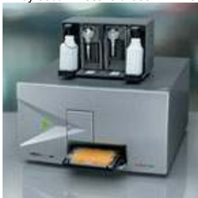
Fig. 1 - Multi-plate reader used for the determination of the DPPH scavenging activity
